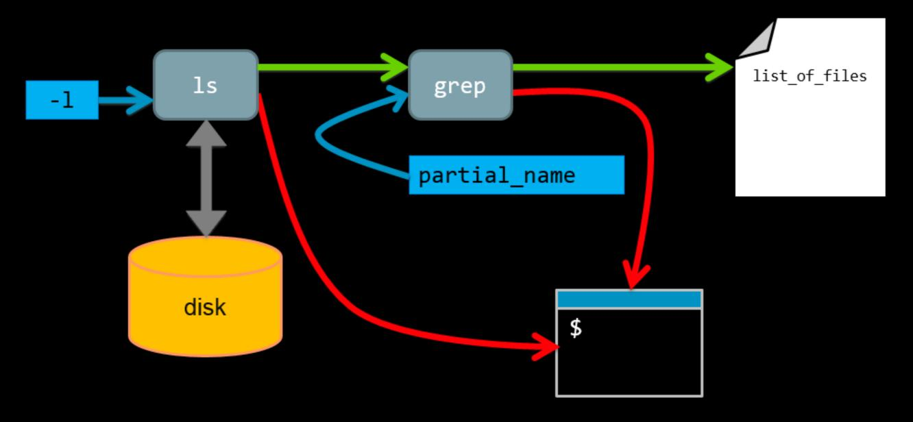
We have piped ( ) the stdout of one command into the stdin of another command!
